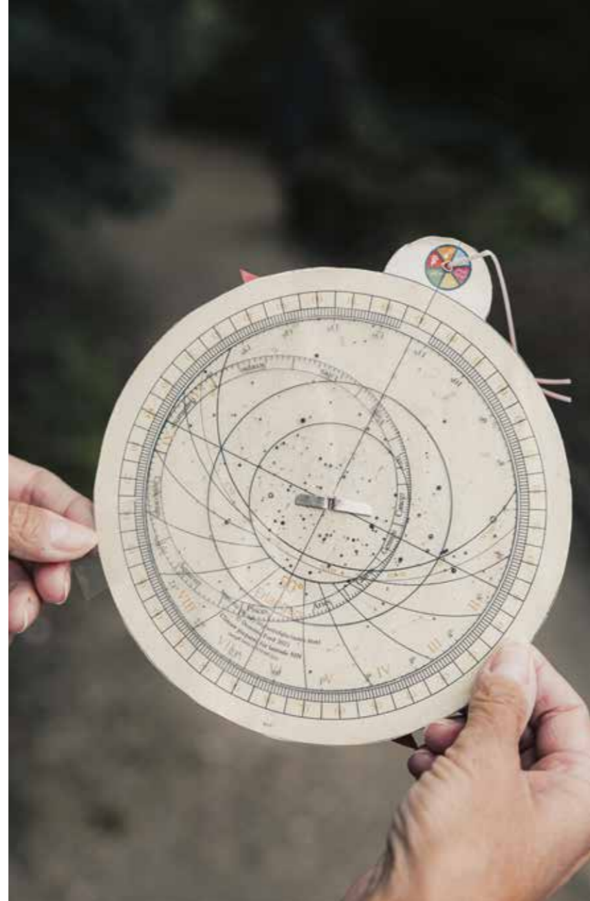
Paper model of an astrolabe calculated for the latitude of Erlangen. It was created for the Humanities Festival "Glimpses into the Future" in 2021.
